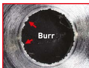
Cutting off without chamfer with burrs
