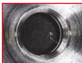
Cutting off after chamfering
